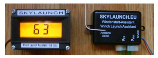
Since winch launching has been invented winch drivers need to estimate the launched glider's speed at a far distance and have to adapt the throttle position to various glider types, characters of pilots and wind conditions. Especially light gliders, long launch runs, strong wind, bad powertrain properties and Dyneema cable with few sag make it hard to launch at optimum and save speed. Even cable tension and cable speed controlling systems cannot ensure proper air speed.
