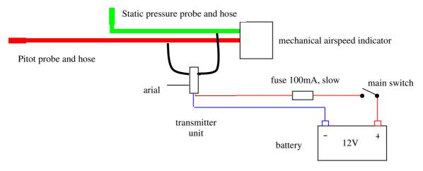
not necessarily fix the transmitter's housing. Arial wire parallel to the glider's lateral axis (wing), install the wires properly and fix them.
